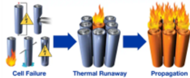
Figure 1: Diagram depicting a cascading thermal runaway event.
